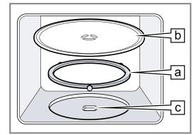
2. Engage the turntable **b** in the drive **c** in the centre of the cooking compartment floor.
