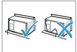
Insert the appliance into the unit and move it to the right.
