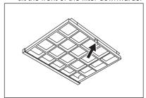
3. To install a new filter, perform the same steps in reverse order. In any case, it is necessary to replace the filters at least every four months.
