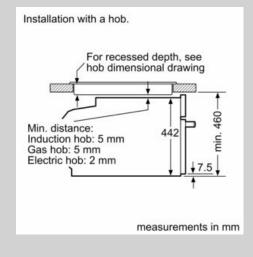
If the compact appliance will be installed underneath a hob, the following worktop thicknesses (including substructure if necessary) must be taken into acccount.
