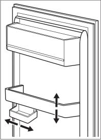
This model is equipped with a variable storage box which can be moved sideways.
